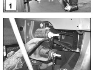
**2d**) Remove the bolts securing the rear shackle to the hanger (**Photo 2**). Carefully lower the leaf spring.
